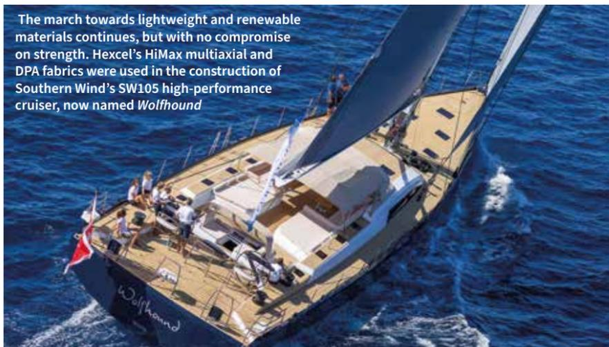
The march towards lightweight and renewable materials continues, but with no compromise on strength. Hexcel's HiMax multiaxial and DPA fabrics were used in the construction of Southern Wind's SW105 high-performance cruiser, now named *Wolfhound*
